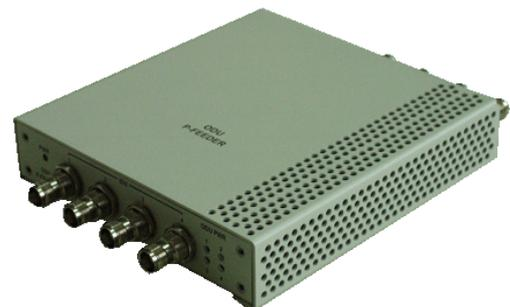
received from an external source. Each ODU Power Feeder unit can serve up to four High Power ODUs. Up to three ODU Power Feeder units can be installed in a 1U high Power Feeder panel.
